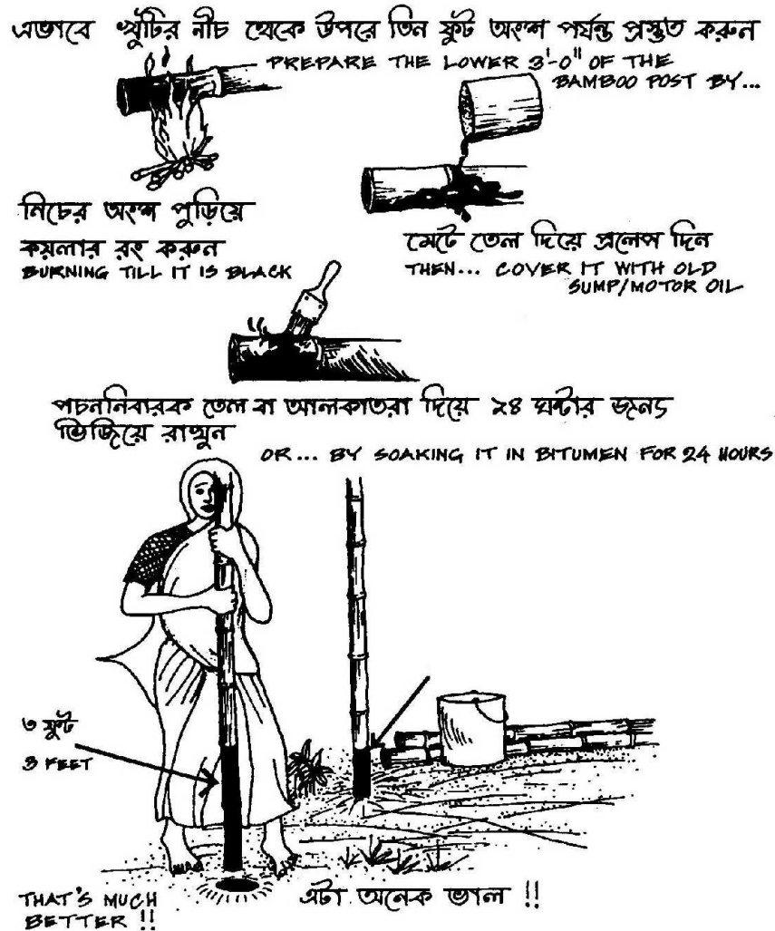
Figure 7: Inexpensive treatment method for bamboo post base (Ahmed, 1994, adapted from Chisholm 1979)
